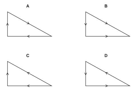
14 Two rigid steel beams XY and YZ are fixed at their lower ends and are hinged at Y. Each beam is inclined at  $50^{\circ}$  to the horizontal, as shown. A weight of  $4.0 \times 10^4$  N hangs from Y. The structure is in equilibrium.
